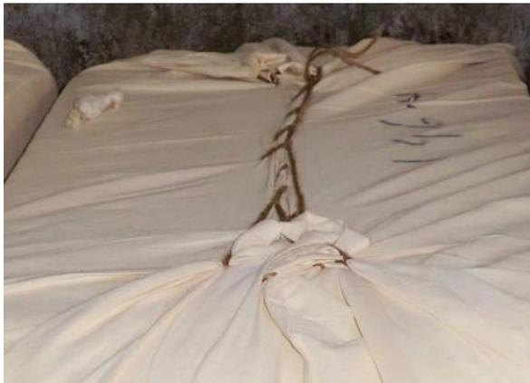
Some ginneries use cotton fabrics to cover bales, but are unaware that jute strings used for tying cause contamination
