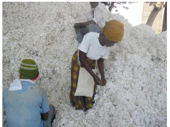
Sorting of contaminants at feeding point reduces contamination
