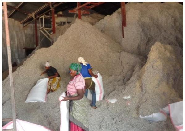
Polypropylene used for packaging seeds can easily contaminate lint if the ginning hall is not separated from seed store
