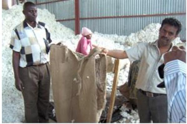
worn-out jute bags used to transport cotton, cause threads to drop in the heap
