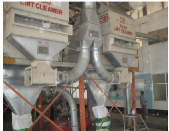
Installation of both pre and post cleaners reduce contamination
