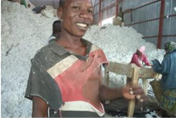
Torn clothing worn by cotton handlers causes threads to drop in the heap which mixes with the cotton and causes contamination
