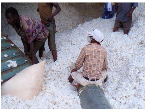
Insufficient number of workers engaged in segregating contaminants at the feeding point
