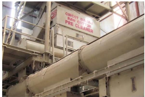
Raw cotton pre-cleaner and lint cleaner machines are installed at the ginnery. Pre-cleaners remove impurities from seed cotton and lint cleaners reduce trash and contaminants and improve fibre quality
