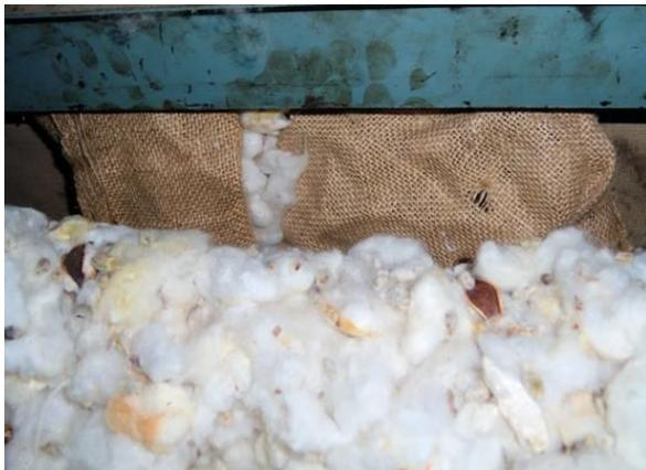
A jute bag is seen stuck in a DR machine during the ginning process. This will contaminate cotton quality. Cotton seeds are not properly being separated from the lint due to poor maintenance
