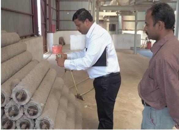
Grooves made on worn-out leather-clad rollers for double roller machines inside the ginnery result in pieces of remnants to mix with the cotton and cause contamination
